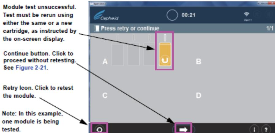
2. If the **Continue** arrow at the bottom of the screen is pressed when there is an unsuccessful module test displayed, the Confirm continue screen will appear.
