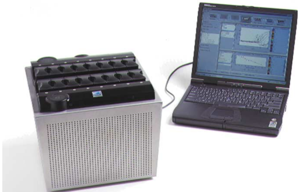
Figure 2: The portable Smart Cycler TD. Real-time PCR assays can be conducted at remote/field locations using the Smart Cycler. The Smart Cycler processing block has 16 independently-controlled reaction sites (I-CORE modules) allowing different cycling parameters to be run simultaneously.
