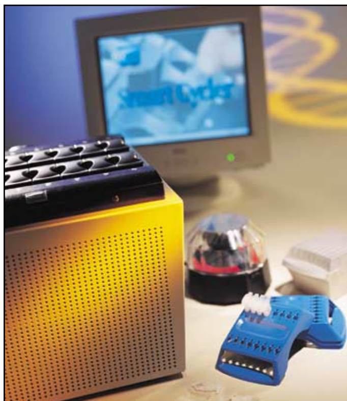
Figure 3: Smart Cycler for real time PCR. The system allows 16 samples run at the same time. The run is completed in 30 minutes.
